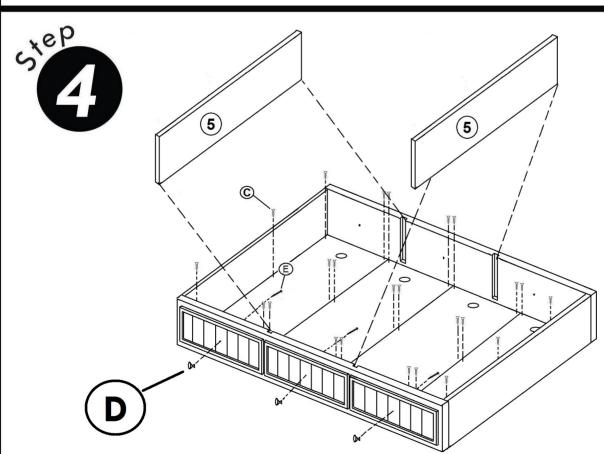
Place Base Boards over Slats. Tighten using CSK screws. Place Dividers into slots.
